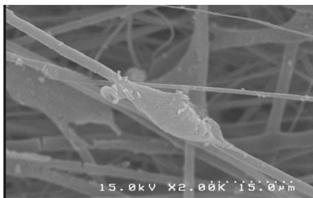
Fig. 12 SEM micrographs of HFSCs seeded on PLLA for 1 day showing the cell–fiber adhesion between the HFSCs and the PLLA fibers. Scale bar=15 \mu m
